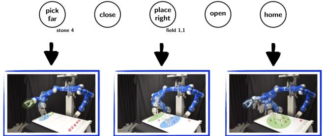
Fig. 2: A possible sequence of terminals produced by the attribute grammar and three of the corresponding primitives.
