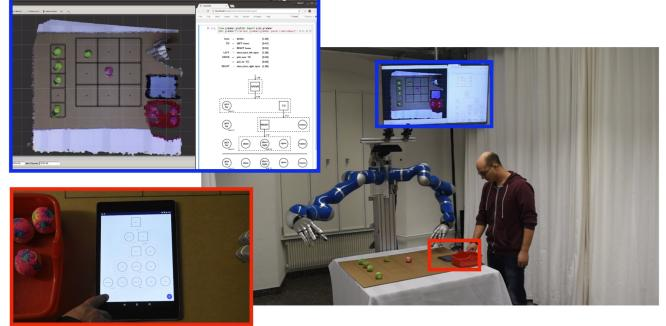
Fig. 1: Playing tic-tac-toe against the robot. The robot executes a sequence of primitives, picking up a stone and placing it on an empty field. The primitives correspond to terminals in an attribute grammar. The sequence of terminals was produced using the general evaluation scheme for movement primitive tasks presented in this paper.
