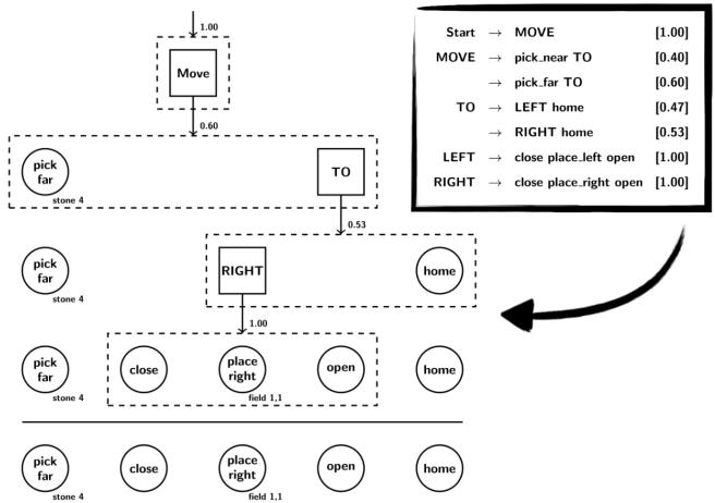
Fig. 3: A parse tree as produced by the attribute grammar for making a move in a game of tic-tac-toe. The grammar applied the general evaluation scheme for movement primitive sequencing as presented in this paper.
