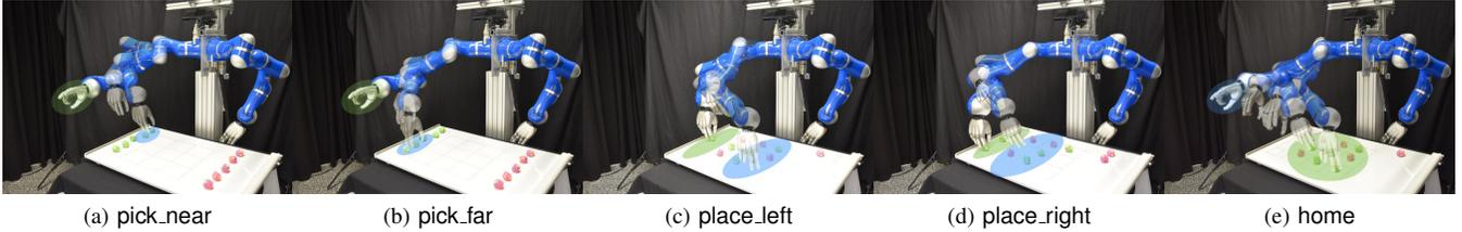
Fig. 3: The five arm primitives used in the sequences, representing turns in the tic-tac-toe game.
