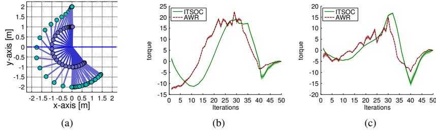
Figure 4: (a)Two-Link Pendulum Swing-Up solution found by ITSOC. (b,c) The resulting torque trajectories are shown for the ITSOC algorithm as well as for the value-based AWR method. AWR only found a suboptimal solution that exhibits considerably more jerk in the torque profile.
