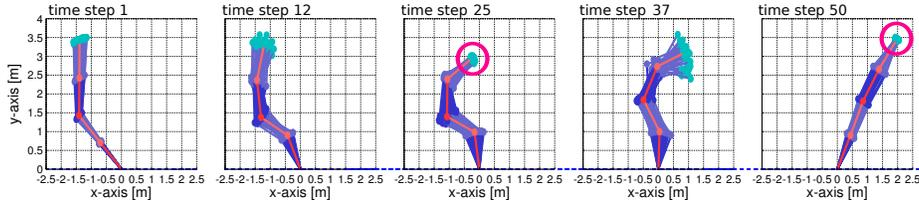
Figure 6: Illustration of the resulting postures for the via-point task in task space. The non-linear planar arm has to reach the via-points at  $t = 25$  and  $t = 50$  illustrated by pink circles. The plot shows for each time step samples from the resulting distribution of postures. The mean of the postures is shown in red. The robot managed to reach the via-point while exhibiting a significant amount of variance in joint space.
