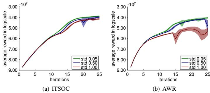
Figure 7: Evaluation of the robustness of ITSOC and AWR to deviations of the initial state. We varied the standard deviation of the initial joint configuration from 0.05 to 1.0. While the learned policies of ITSOC only slightly degrade, the AWR algorithm could not handle the situations with a large deviations in the initial state.
