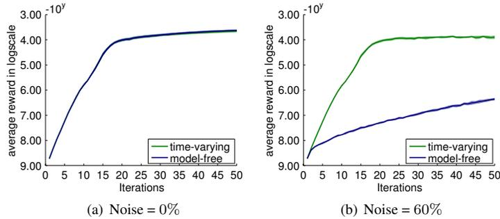
Figure 5: Comparison of ITSOC with learned models and without learned models where we use a single sample estimate for the expectation of the next features, which results in a bias in our optimization. The evaluations are done for different noise levels of additive control noise. Model-based ITSOC shows the best performance while the biased version of ITSOC quickly degrades with an increasing noise level. Note that all plots are in log-scale for the y-axis.
