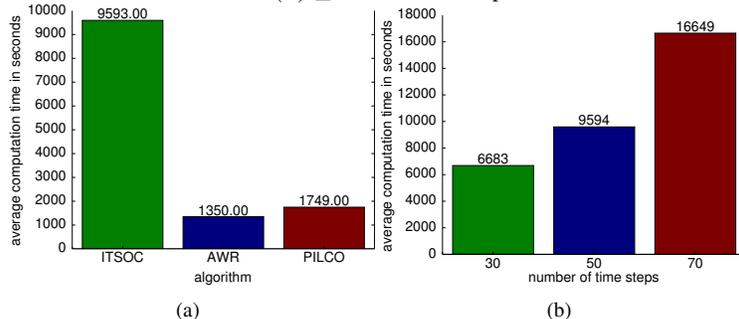
Figure 9: (a) Comparison of the computation time of the different algorithms. The bars show the average time needed for 50 iterations on the quad-link reaching task. (b) Computation time of ITSOC for an increasing number of time steps.
